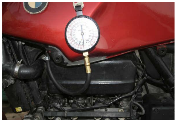
Testing the pump pressure
