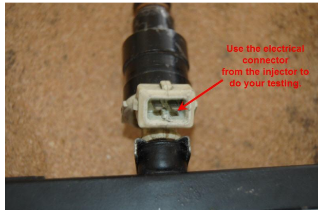
Testing the coil of the fuel injector
