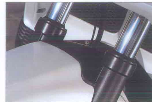
Strong and reliable: The fork stabilizer for optimum handling at all speeds.
