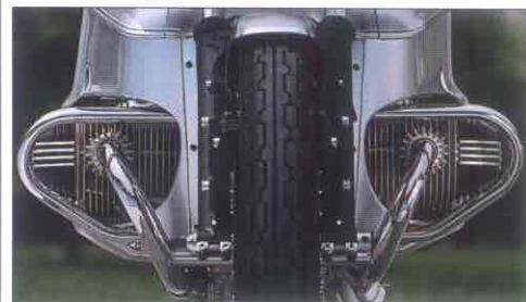
To this day there's no better engine for motorcycles up to 60 bhp than the two-cylinder. And one of the best two-cylinders is certainly the Boxer. The reasons: ideal thermal stability, low weight, low center of gravity, long running life, simple maintenance, supreme torque, outstanding flexibility and a perfect balance of all forces. Add to this the classic looks of the Boxer and you have the perfect concept.
