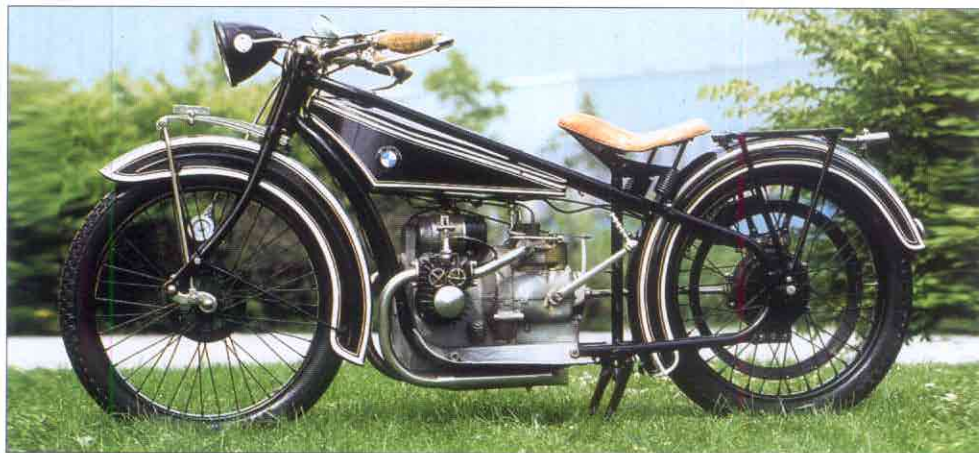
The original: the R32 launched by BMW in 1923. The first rendition of BMW's typical Boxer design.
