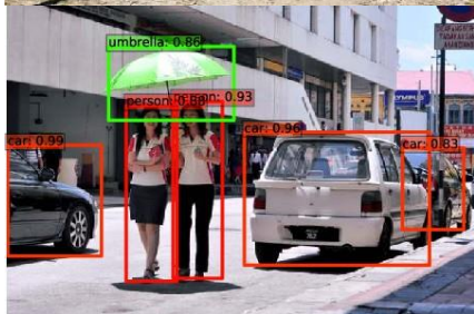
Figure 6.2: Examples of object detection with the Single-Shot Detector [Liu et al., 2015].
