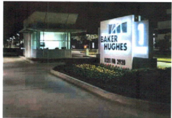
Figure 14. A well-balanced lighting system between the interior of the guardhouse and the exterior surveillance lighting. Note that the guard station is not staffed and the guardroom is lit for effect (to give the appearance of human presence (Photo courtesy of OSS – Law Enforcement Advisors ® )
