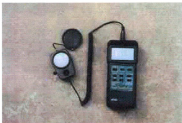
Figure B1. Typical Illuminance Meter. (Provided courtesy of OSS – Law Enforcement Advisors®)
