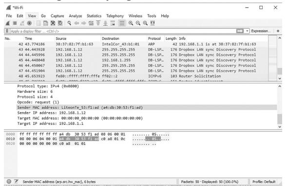
After you record some network data, it's time to take a look at the captured packets. The captured data interface contains three main sections: the packet list pane, the packet details pane, and the packet bytes' pane.
