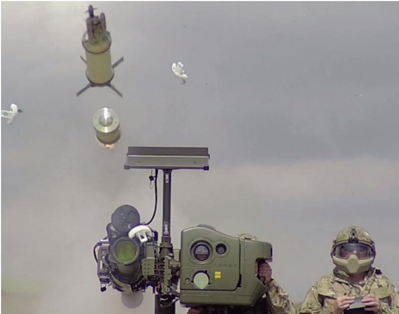
**Figure 2.57** A Thales UK Lightweight Multiple Launcher – Next Generation (LML-NG) firing a STARStreak high-velocity surface-to-air missile. This type of light guided missile launcher is often considered a ‘crew-portable air defence system’ (CREWPADS) (source: Thales UK).
