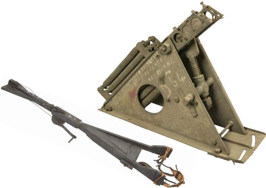
**Figure 2.61** Two light projectors. *left: a Leach–Gamage Catapult, which used elastic rubber tubing to store mechanical energy. Right: a West Spring Gun, which employed several coiled springs to achieve a similar effect [not to scale] (sources: Imperial War Museum; Australian War Memorial).*
