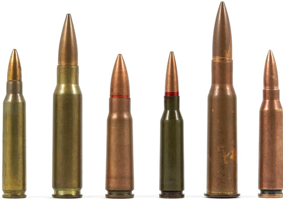
**Figure 2.17** Dominant rifle cartridges in military service globally, L-R: 5.56 × 45 mm; 7.62 × 51 mm; 7.62 × 39 mm; 5.45 × 39 mm; 7.62 × 54R mm; and 5.8 × 42 mm (source: Jack Dutschke/ARES).
