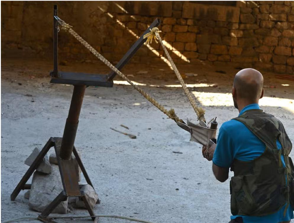
**Figure 2.62** An improvised light projector, used to project craft-produced high explosive munitions in Syria (source: AFP).
