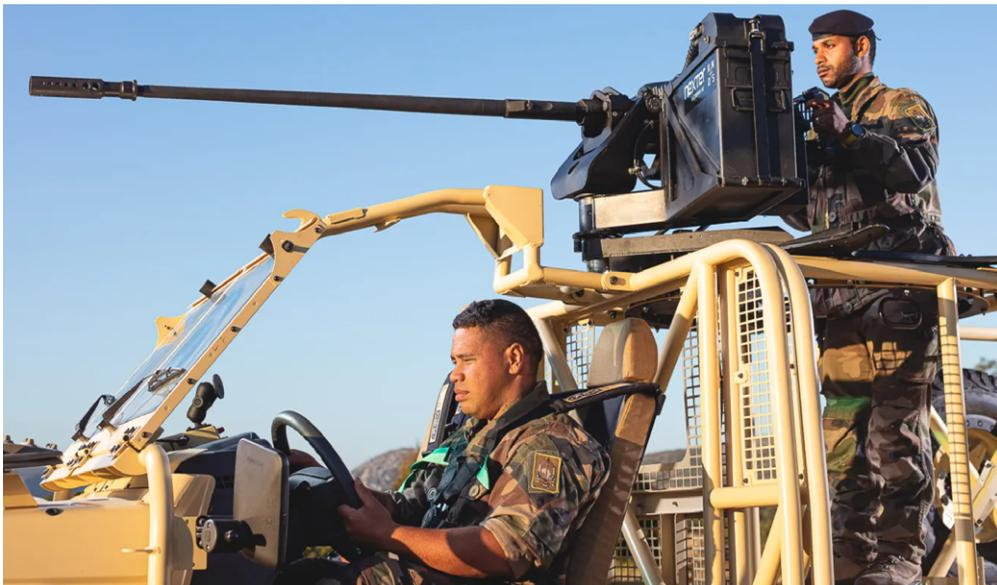
**Figure 2.47** A Nexter P20 (20 × 102 mm) light cannon, mounted on a military vehicle. In recent years, light cannons such as this have been positioned as replacement armaments for .50-calibre machine guns on light tactical vehicles (source: Nexter).
