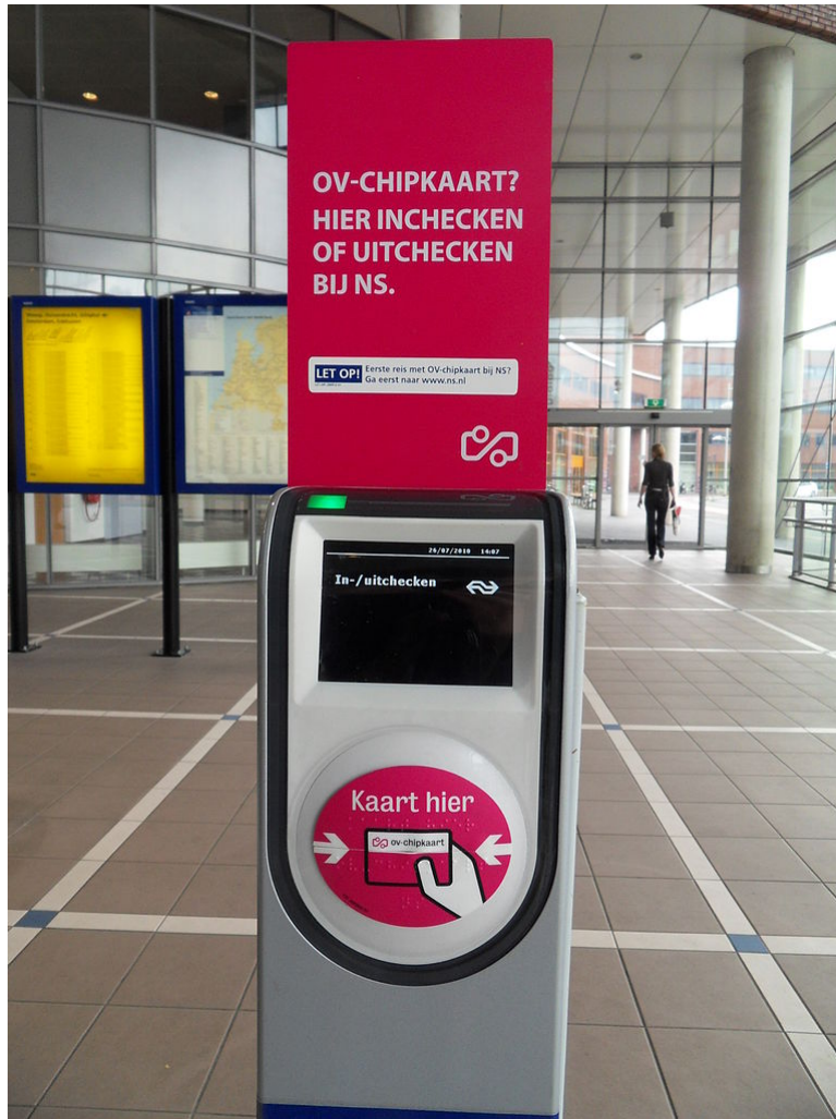
Figure 2.3: RFID ticket validator for a barrierless system in the Netherlands [5]
