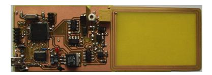
Fig. 1. Our stand-alone RFID emulation device.
